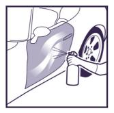
Ensure that the surface is dust free. Apply at least 1 hour after the last coat of the base-coating has been applied. On worn coatings, a ph-neutral wash and use of  $0^2MPREP$  is recomended.
